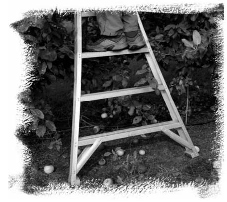
worker grabbed the ladder with one hand and was left hanging. The hand was injured as well as the back. The worker attributed the injuries and severity to the weight of the bag, the slippery conditions and frosty weather. The three-legged ladder was set with the third leg to the outside of the tree.
